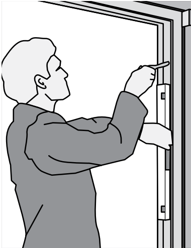
Fig. 22: Fix frame in opening
